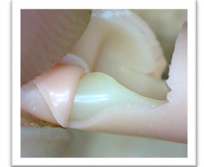
Inspection of latex tube delamination
